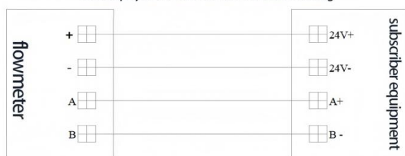
With display and 4-wire 485 communication wiring
