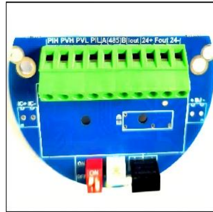
Two-wire system 4-20mA current output integrator with display (two-wire to four-wire)
