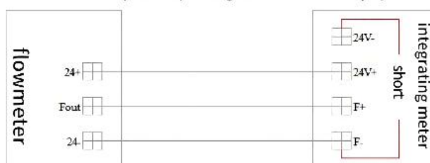
Three wire pulse output integration device with display
