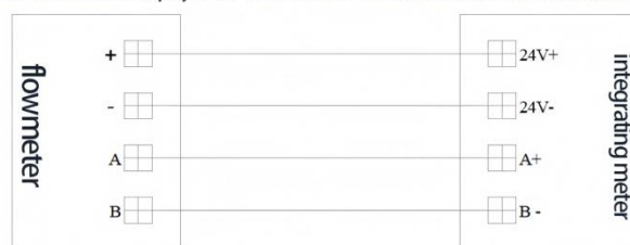
Instrument with display and 4-wire 485 communication for cumulative calculation
