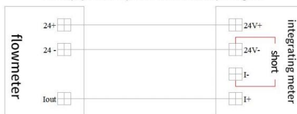
With display three wire system 4~20mA current output integrator
