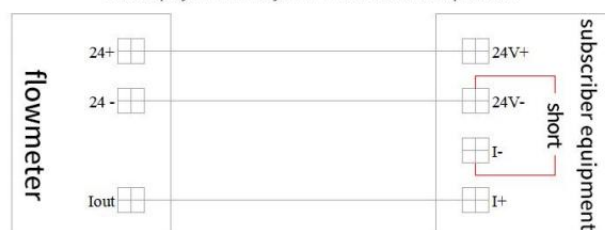
With display three-wire system 4~20mA current output cable
