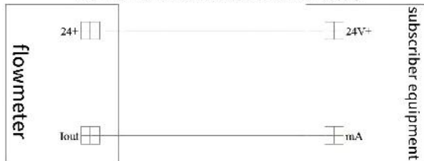
Two-wire 4-20mA current output cable with display
